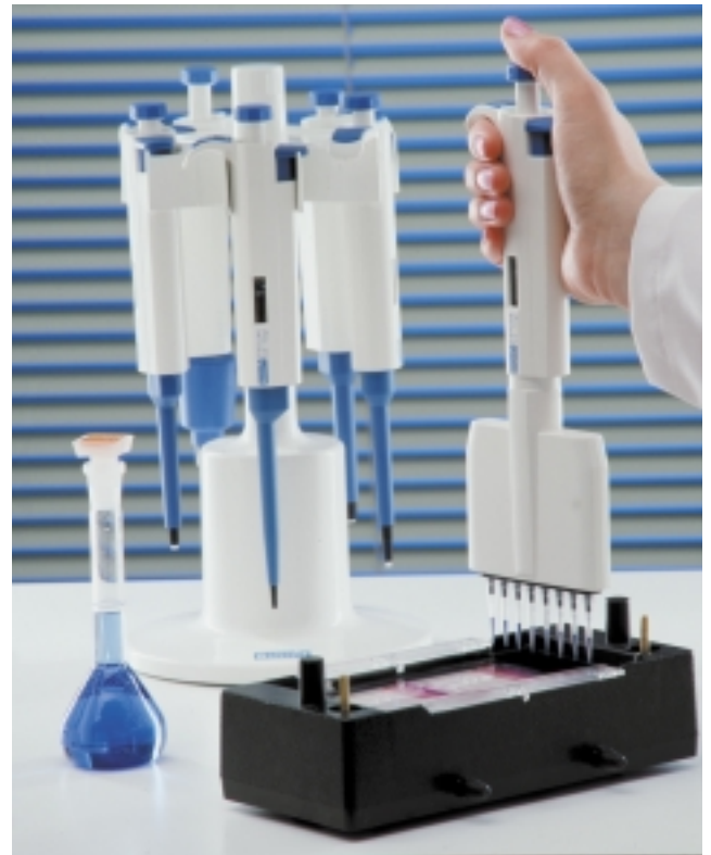
Fig 1. The major design of mechanical pipettors on the market resemble each other. However, some manufacturers have added special features, like Biohit has filters on tip cone of the pipettor to prevent contamination.
