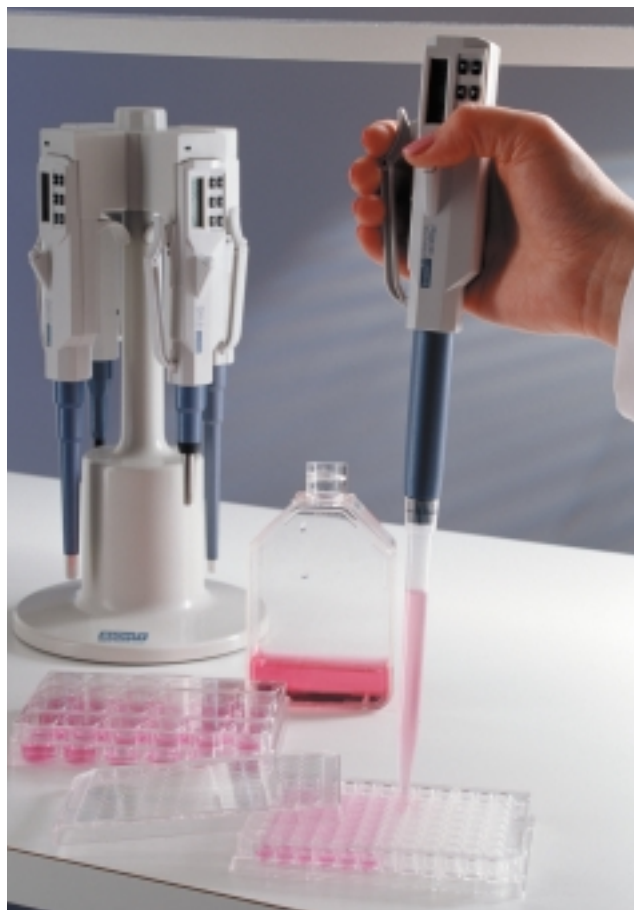
Fig 3. Electronic pipettors diminish workload, guarantee high reproducibility and accuracy, and reduce the person-to-person variation.
