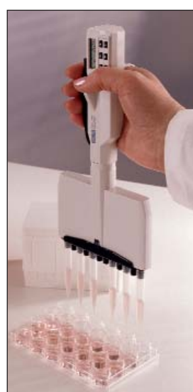
Figure 2. Electronic pipettors can be used effectively and accurately in dispensing to various cell culture plates.
