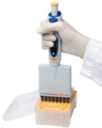
Figure 3 The Biohit Optiload system, featuring spring loaded tip cones, allows pipettor tips to be picked up with a constant force. This, in turn, guarantees even tip sealing and sample pick-up and reduces tip ejection force considerably, compared to conventional pipettors.
