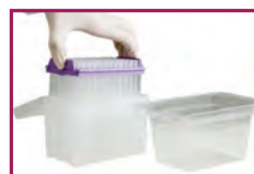
Take the tip tray from the Refill Pack and put it into the empty tip box.
